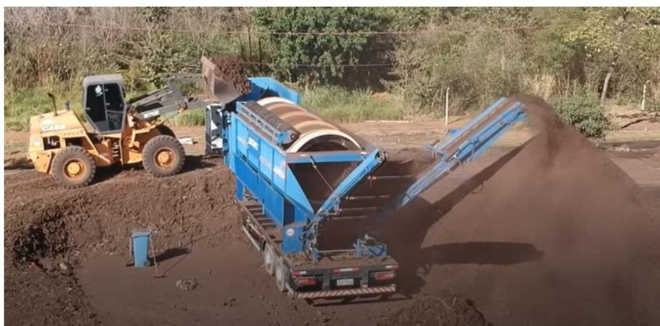
Figure 8: The compost screening operation.
