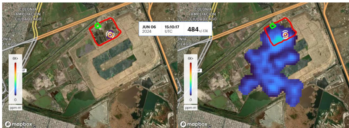
Figure 1 - PC-BP site and overlay of methane plume (blue). Origin of plume is the orange point encircled in purple, PC-BP outlined in red, PCH-CDMX outlined in green. Source: Adapted from Carbon Mapper (Carbon Mapper, Inc., n.d.).
