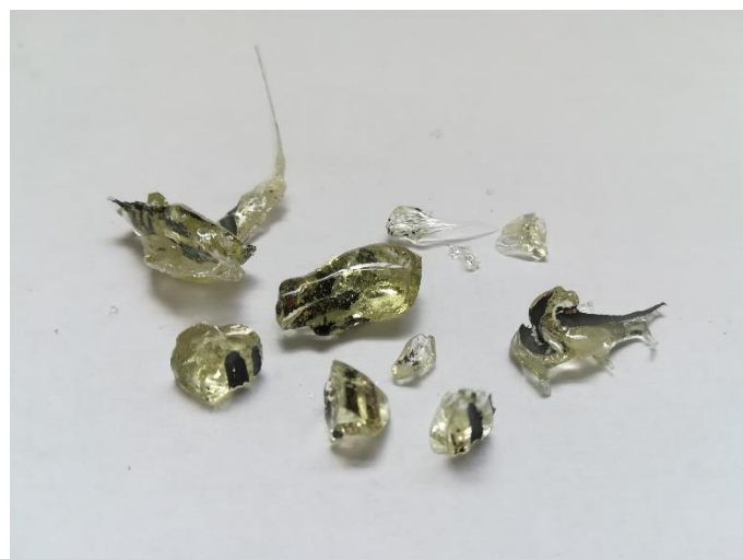
Fig. 4. EXP1. Final result of the experiment. Transparent, pale green-yellow glass, including some iron scale from the scrapper tool (in the large fragment, slightly left of centre).
