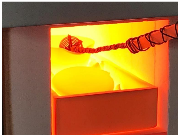
Fig. 3. EXP1 (step 6 of the recipe). Scum removal from the glass melt using an iron tool.
